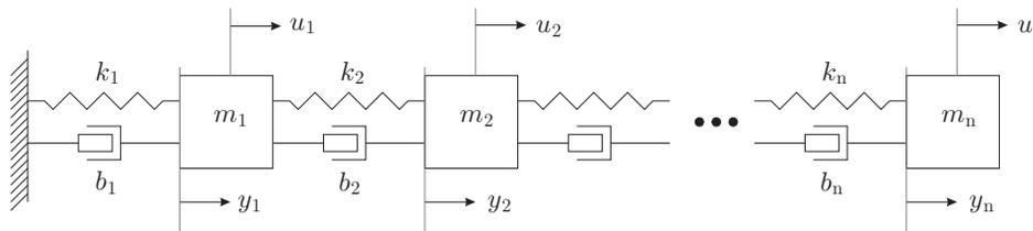
The masses have mass 1, the spring constants are all 0.8, and the damping constants are all 0.32.
